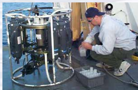
A CTD is attached to a metal frame called a rosette, or carousel, along with numerous water sampling bottles and when deployed, provides information about the composition of the water column. Image courtesy of NOAA.
